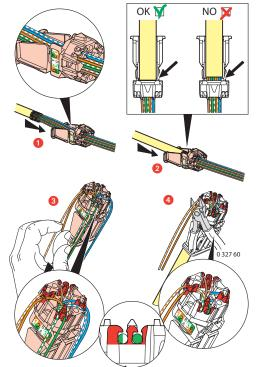
Spreading the cables and positioning the sleeve firmly in the spreader ensures that a pair-breakage distance of 13 mm is kept between pairs, as required by the standard.
